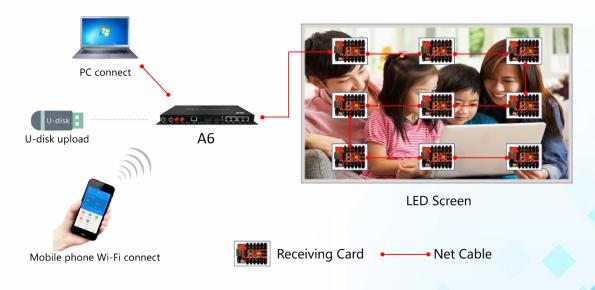
3. Real-time picture synchronization display: The play box is connected to the sync source through the HDMI high-definition video line, and the sync picture is automatically scaled without any setting.
